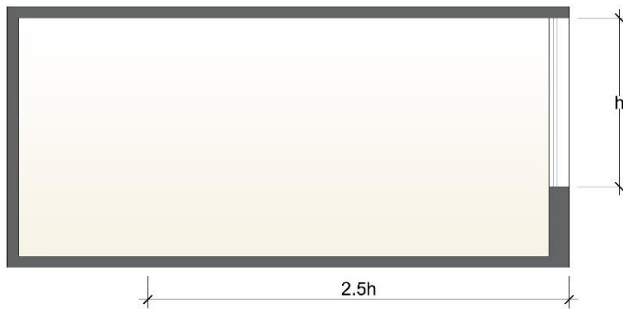
Figure 10: Daylight penetration extent in a space.
